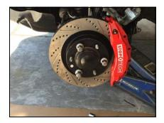
Slide Caliper over rotor with the bleed screws facing up.
