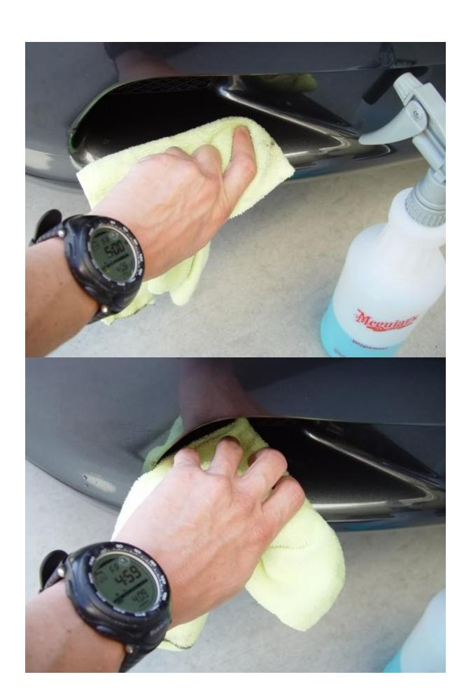
Place your lip on a soft surface such as plastic, grass, etc. so as not to scratch it up. Apply 3M adhesive tape to the following areas. I personally recommend one thin strip in each area where the lip will rest just below the vents. Apply 2 thin strips, one behind each other, the entire length of the area where the lip will sit just in front of the lower bottom grille. Remove the protective backing of tape; exposing the tape itself for mounting the lip on the bumper.
