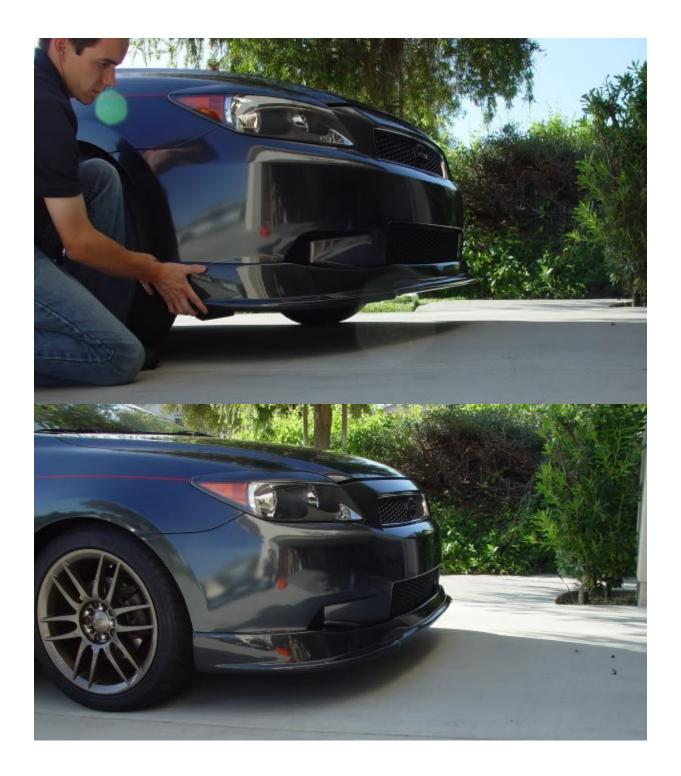
Once you pull the ends of the lip into the wheel wells, you are ready to screw them into place. If you notice a lack of space while screwing the lip into the bumper, simply turn your wheels the opposite direction.
