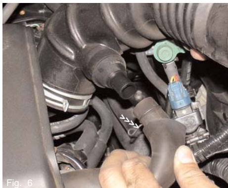
Fig. 6 Use a pair of pliers to depress the wire tension clamp located on the crank case breather hose. Pull the breather hose off the air intake port as shown above.
