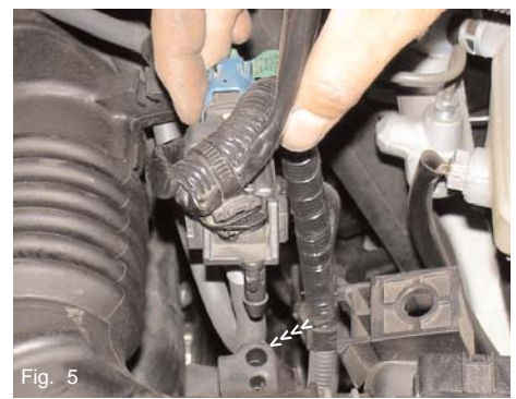
Fig. 5 Pull the entire vacuum switching valve from the rubber saddle on the air intake duct used to secure the vacuum switching valve.
