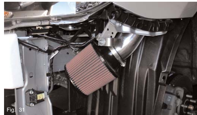
The filter is placed on the end of the secondary intake and the clamp on the filter neck is fastened to secure the filter in place. Align the entire intake for the best possible fit. Once proper clearance has been made through out the length of the intake, continue to tighten all nuts, bolts and clamps.
