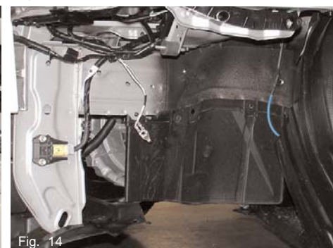
Fig. 14 Remove the entire front bumper by removing all bolts and plastic clips holding the bumper in place.
