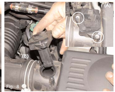
Fig. 8 Unscrew the two screws that secures the mass air flow sensor to the sensor housing (A). Pull the mass air flow sensor up and out of the sensor housing as shown above (B), to be used later in the instruction.
