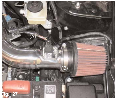
The MAFS is pressed into the adapter and sitting flush(A). Make sure that there are no air leaks in the sensor. The Cold air intake can also be converted into a short ram as seen in this picture. Simply, press the air filter over the end of the primary intake(B).
