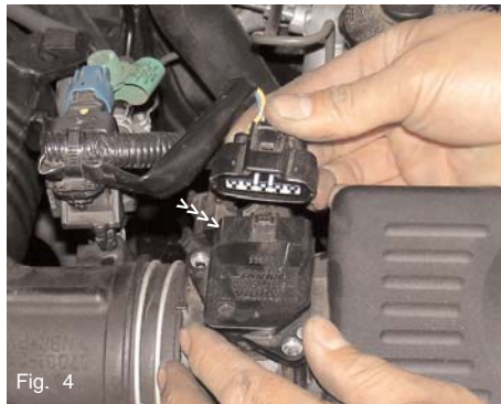
Fig. 4 Disconnect the mass air flow sensor electrical harness from the sensor.
