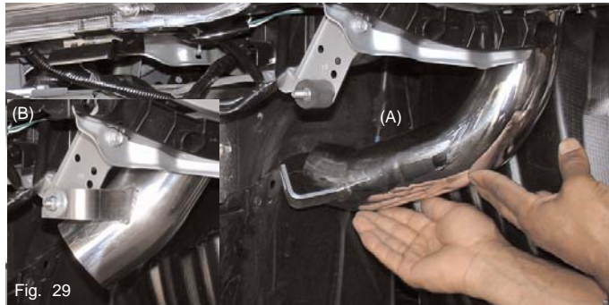
The secondary intake system is inserted through the bumper area. Close attention is placed on the resonator opening when going up and into the engine compartment(A). Once the intake has been slipped up and into the engine bay, the top end is butted up against the primary intake. Now, align the bracket to the vibra-mount stud and use the fender washer and flange nut to secure them(B).
