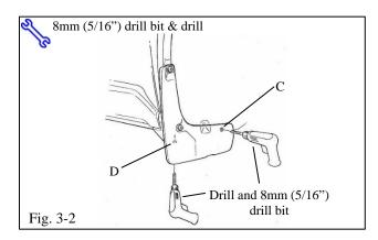
(b) While holding the part up and into body panel, use the part as a template to drill 8mm (5/16") holes in locations C and D (Fig. 3-2).
