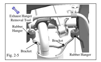
(f) Pry the two front muffler exhaust brackets loose from the rubber hangers. (Fig. 2-4)
