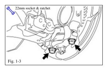
(i) Remove the two bolts from the lower ball joint assembly (Fig. 1-3). Retain the bolts for reinstallation.
