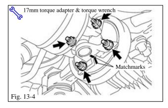
(d) Install the propeller shaft to the rear differential using the four nuts. Tighten the nuts (Fig. 13-4).
