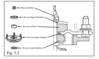
(b) Install the lower retainer, cushion, upper support and upper retainer to the piston rod (Fig. 3-2).
