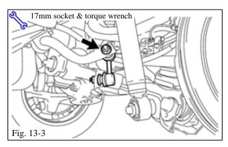
(b) Install the stabilizer link bolt into the stabilizer bar assembly and attach the OE nut (Fig. 12-3).
