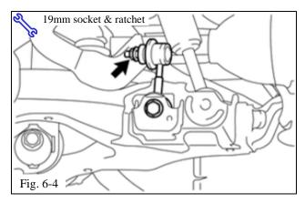
(c) Install the stabilizer link bolt into the stabilizer bar assembly and attach the OE nut (Fig. 6-4).
