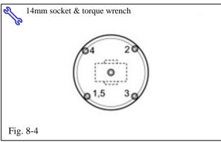
(e) Tighten the four upper shock assembly nuts in a crisscross fashion (Fig.4-5).
