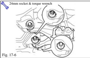
(q) Tighten the lower control arm bolts (Fig. 17-6).
