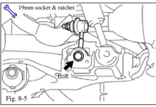
(g) Install the stabilizer bar link to the lower control arm and tighten the bolt (Fig. 8-5).
