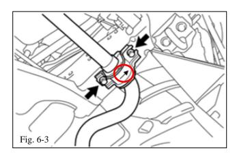
CAUTION: Make sure to install the brackets so that the arrows imprinted onto the brackets face the front of the vehicle (Fig. 6-3).
