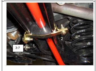
(2) Place outside edge of clamps at this point on the beam axle. (Fig. 3-5)
