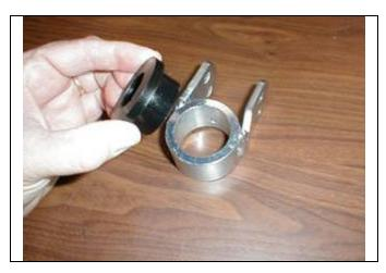
(c) Insert two shock eye bushings (do not grease the outside of the bushings) from each side into the shock eye.
