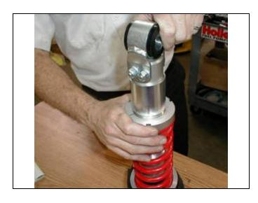
(n) Apply a pre-load to the spring by turning the spring perch so that <sup>3</sup>/<sub>4</sub>" or 20 mm of threads are showing below the spring perch.
