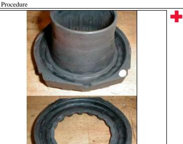
(f) Remove the skirted area from the upper spring insulator using tin snips or a box cutter.
