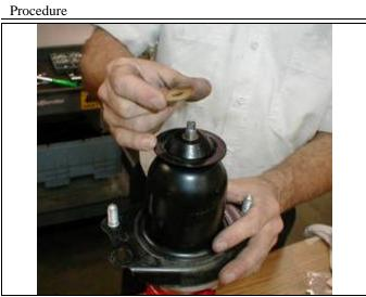
(m) Install a 3/8-24 locknut and cup washer on the shock shaft.
