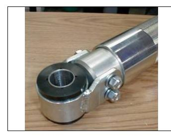
(e) Assemble the lower shock eye to the shock body using two M8 x 1.25 x 60 bolts, two M8 x 1.25 locknuts and four M8 flat washers.
