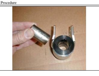
(d) Grease one of the 1" OD shock eye spacer tubes with chassis lube and insert it into the bushings inserted in Step 13-C.
