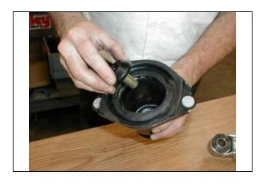
(j) Install one suspension support grommet, with a 9/16" OD spacer tube inserted, into a rear spring front bracket sub-assembly from the bottom. Make sure the upper insulator is seated properly.
