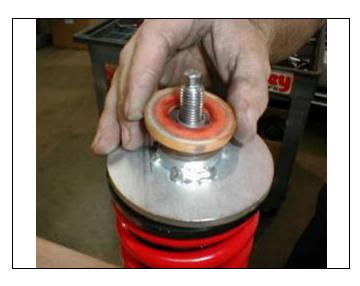
(g) Install the factory front suspension support dust seal over the protrusion on the top of the upper bearing adaptor.
