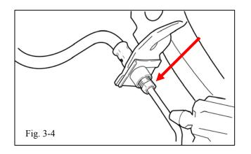
(b) Place a drip tray directly below the inboard brake line connection. This connection is where the rubber hose attaches to the steel brake line as shown in (Fig. 3-1).
