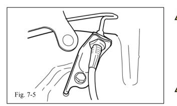
(c) The orientation of the banjo fitting should be such that the stainless steel brake hose is pointing as shown (Fig. 7-3).
