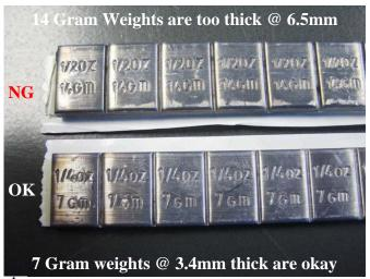
CAUTION: These wheels MUST be balanced using the thinner 7 gram weights. The thicker 14 gram weights will contact and rub the paint off the calipers.
