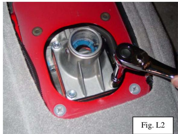
**M. Install TRD Shift Lever Assembly**
