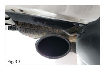
(f) Remove the protective covering from the exhaust tip.
