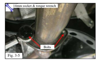
(e) Make sure the muffler flange is lined up to the converter assembly flange. Reinstall the two (2) OE bolts and tighten them to 48 N-m (35 lb-ft) (Fig. 3-5).
