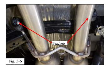
(g) Attach the two hanger brackets of the TRD center muffler assembly front pipes to the existing rubber hangers and rods on the vehicle frame (Fig. 3-6).
