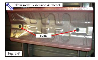
(i) Locate the body side heat shield on the rear deck above the original tailpipe. Remove the two bolts holding the body side heat shield to the rear deck and remove the heat shield (Fig. 2-8).
