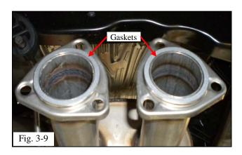
(1) Install the two new gaskets, supplied in the kit, on the TRD center muffler assembly rear outlet pipes (Fig. 3-9).
