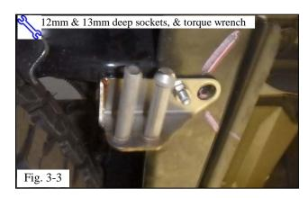
(c) Locate the larger hole on the exhaust bracket to the rivet head while engaging the bracket slot onto the vehicle cross-member. Insert the 8mm bolt supplied in the kit into the smaller hole from above (Fig. 3-3).
