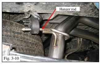
(m) Attach the hanger rod of the TRD RH tailpipe assembly to the rubber hanger on the vehicle frame (Fig. 3-10).
