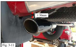
(n) Align the RH tailpipe with the RH outlet pipe on the muffler and install the nuts and bolts. While tightening the bolts, set a gap of 30±5mm between the exhaust tip and the rear side panel (Fig. 3-11).
