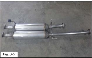
(f) Reinstall the rubber hanger removed in Step 2(h) to the rear hanger of the muffler assembly (Fig. 3-5).
