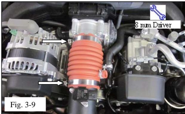
(i) Tighten both hose clamps securing the TRD coupler hose to the throttle body and TRD Air Box. (Fig. 3-9)
