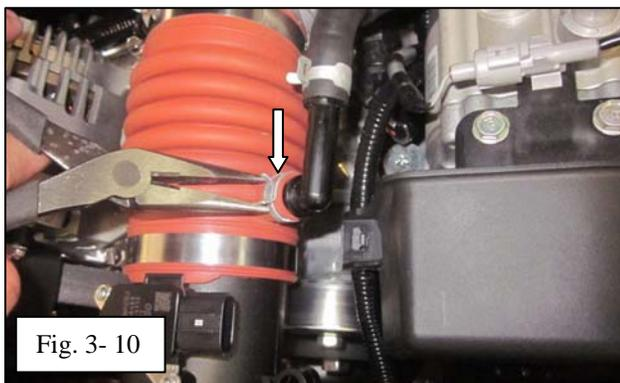
(j) Attach the crank case vent fitting to the TRD coupler hose and secure with spring clamp. A small amount of soapy water will help with the installation. (Fig. 3-10)
