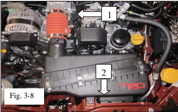
(h) Install the complete TRD Air Box assembly into the engine compartment.
