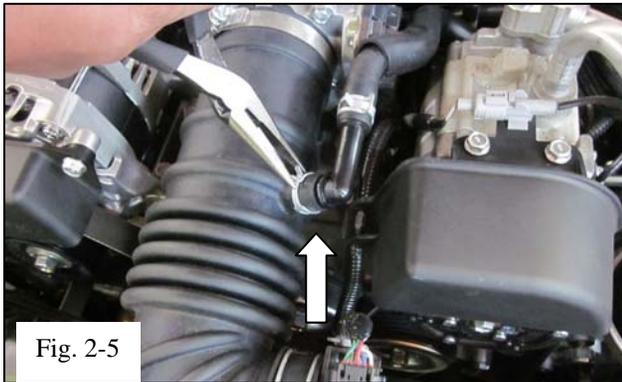
(e) Disconnect the crank case vent hose from the Air Intake Bellows by squeezing the spring clamp. (Fig. 2-5)
