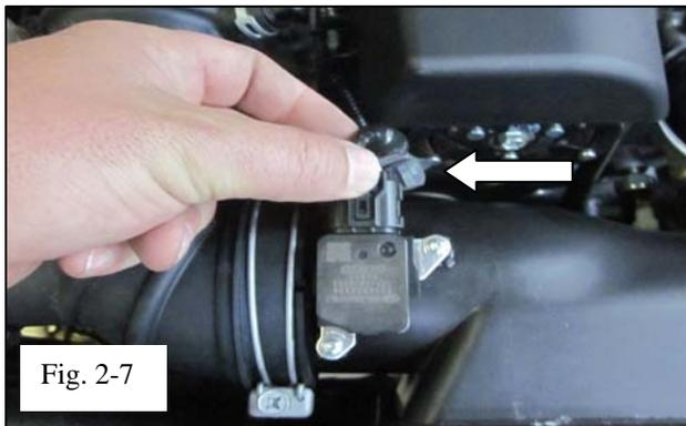
(g) Unplug the MAF sensor and unclip the wiring harness from the OEM Air Box. (Fig. 2-7)
