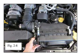
(h) Move the OEM Air Box toward the cowl to disengage from fresh air duct. Remove the complete assembly from engine compartment. (Fig. 2-8)
