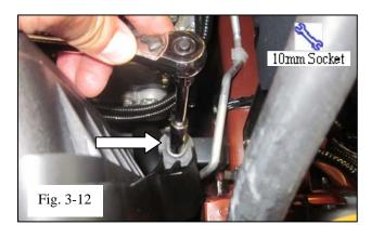
(1) Secure the tab on the TRD Air Box base to the inner fender with the M6 bolt removed from step 2 (c). (Fig. 3-12)
