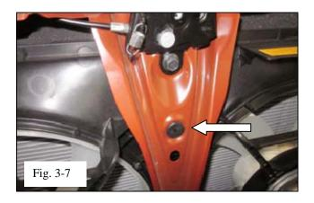
(g) Install the supplied rubber grommet into the circular hole right below the hood release. A small amount of soapy water will help in installing this part. (Fig. 3-7)
