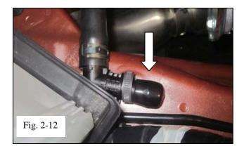
(l) Cap off the fitting on the frame rail with the supplied cap plug. (Fig. 2-12)
