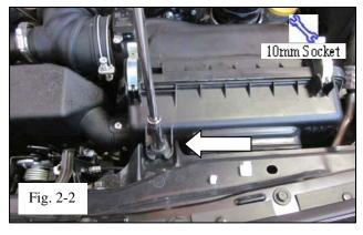
(b) Remove the M6 bolt securing the OEM air box lid to the radiator support. (Fig. 2-2)
