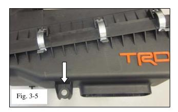
(e) Transfer two of the grommets from the OEM air box to the TRD Air Box. (Fig. 3-5)
