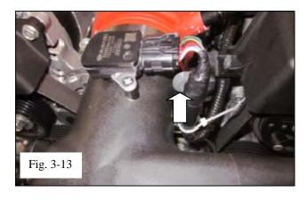
(m) Plug in the MAF sensor wire harness; secure the MAF sensor wire harness to the TRD Air Box with supplied zip tie. (Fig. 3-13)
