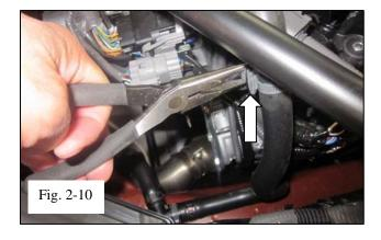
(j) Unclip the Sound Generator tube from the bracket under the passenger strut tower brace. (Fig. 2-10)
