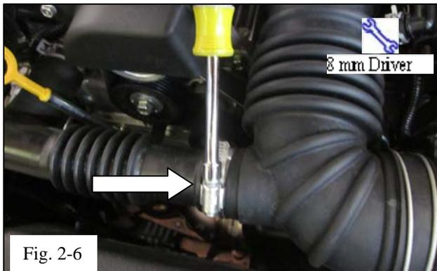
(f) Loosen the hose clamp securing the Sound Generator Tube to the Air Intake Bellows. (Fig. 2-6)
