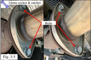
(d) **PPO Only:** Verify the OE gaskets at the two front flanges, located between the catalytic converters and muffler front pipes, are in place before reconnecting the pipes.
