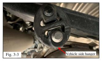
(c) Attach the rubber hanger on the rear of the TRD center muffler assembly to the hanger on the vehicle frame (Fig. 3-3).
