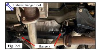
(f) Pry both OE center muffler assembly front pipe hangers loose from the two rubber hangers, located in front of the muffler, and leave the rubber hangers in place on the vehicle (Fig. 2-5).
