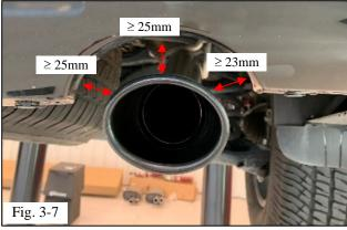
(j) Align the tailpipe with the rear panel so that the sides are even, and the top has clearance as shown (Fig. 3-7).
