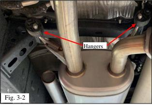
(b) Attach the two hanger brackets of the TRD center muffler assembly front pipes to the existing rubber hangers and rods on the vehicle frame (Fig. 3-2).
