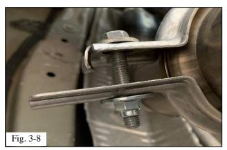
(k) Tighten the V-clamp between the rear of the muffler and the front of the tailpipe (Fig. 3-8). Ensure it is in the proper orientation (Fig. 3-9).
