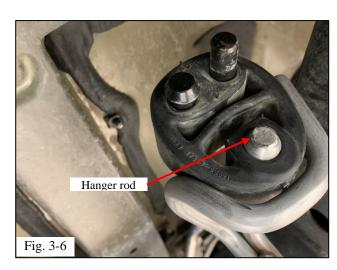
(i) Attach the hanger rod of the TRD tailpipe assembly to the rubber hanger on the vehicle frame (Fig. 3-6).
