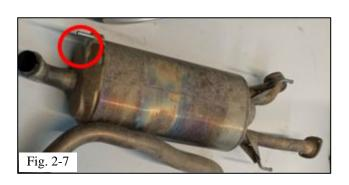
(h) Remove the OE center muffler assembly; remove the rubber hanger from the rear of the muffler (Fig. 2-7).
