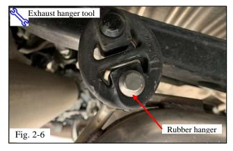
(g) Pry the rubber hanger located at the back of the muffler loose from the vehicle side hanger rod (Fig. 2-6).
