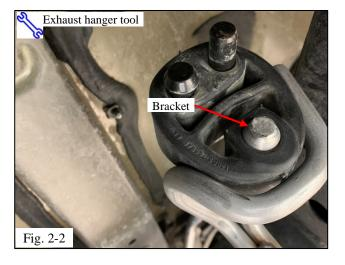
(b) Pry the passenger side tailpipe bracket loose from the rubber hanger (Fig. 2-2).
