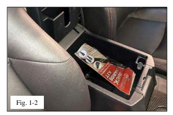
(b) Place the cable charge kit in the console box (Fig. 1-2).
