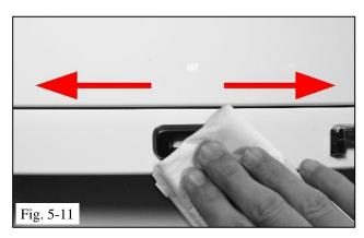
(h) Using a lint-free scratch resistant cloth, press firmly on the emblem cap from the center working outwards to the edges of the emblem cap, to ensure maximum adhesion contact (Fig. 5-11).
