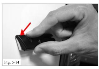
(k) Position the emblem cap over the factory emblem starting from the top edge then downward, ensuring it is centered (Fig. 5-14 & 5-15).
