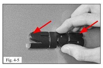
(c) Position the emblem cap over factory emblem starting from the top edge then downward, ensuring it is centered (Fig. 4-5 & 4-6).
