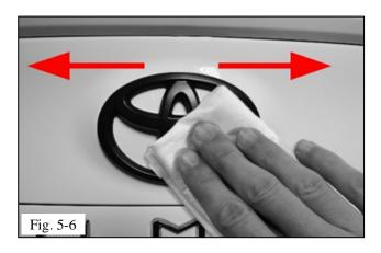
(d) Using a lint-free scratch resistant cloth, press firmly on the emblem cap from the center working outwards to the edges of the emblem cap, to ensure maximum adhesion contact (Fig. 5-6).
