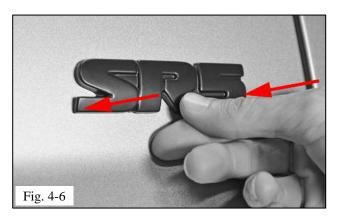
(d) Visually verify that the SR5 emblem cap is positioned evenly over the factory emblem and press lightly to adhere (Fig. 4-6).
