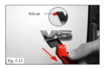
(j) Using the pull tab, pull gently to remove the adhesive liner from the backside of the emblem cap (Fig. 5-13).
