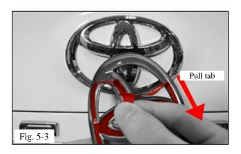
(b) Using the pull tab, pull gently to remove the adhesive liner from the backside of the emblem cap (Fig. 5-3).
