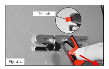
(b) Using the pull tab, pull gently to remove the adhesive liner from the backside of the emblem cap (Fig. 4-4).
