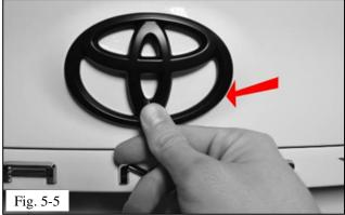
(c) Position the emblem cap over the factory emblem starting from the top edge then downward, ensuring it is centered (Fig. 5-4 & 5-5).
