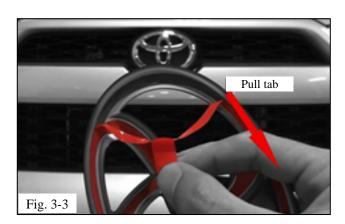
(b) Using the pull tabs, pull gently to remove the adhesive liners from the backside of the emblem cap (Fig. 3-3).
