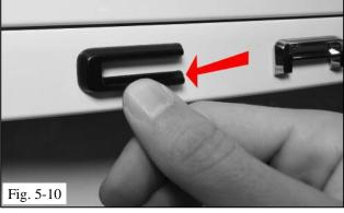
(g) Position the emblem cap over the factory emblem starting from the top edge then downward, ensuring it is centered (Fig. 5-9 & 5-10).
