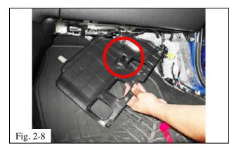
(h) Disengage the foot light connector from the panel (Fig. 2-8).
