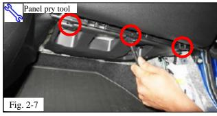
(g) Release the three clips and lower the passenger side under dash panel (Fig. 2-7).
