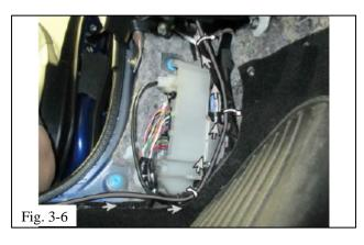
(i) Route the harness along the vehicle harness (Fig. 3-6). Do not attach wire ties yet.
