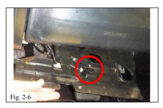
(f) Disengage the foot light connector from the panel (Fig. 2-6).
