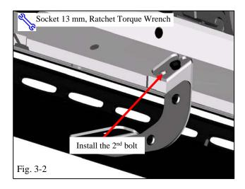
(b) Engage slot of center bracket under head of bolt to secure position (Fig. 3-2). Support with hand while installing the second bolt a minimum of 5 turns.
