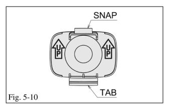
(n) Install the seven (7) bolt covers (7), inserting the bottom tab first (snap facing up) into the running board (Fig. 5-9).
