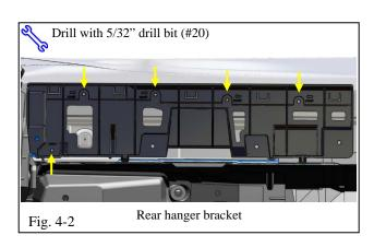
(c) Hold the rear hanger bracket and carefully use the drill with a 5/32" drill bit to drill the 5 marked locations on the hanger bracket (Fig. 4-2).
