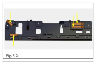
(b) Remove the tape liner tabs located on the rear hanger bracket (Fig. 3-2) and put the part in place.
