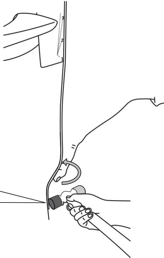
LIGHTLY SEAT DOOR EDGE GUARD STARTING AT THE BOTTOM MOVING UPWARD TO ORIGINAL STOPPING POINT.
