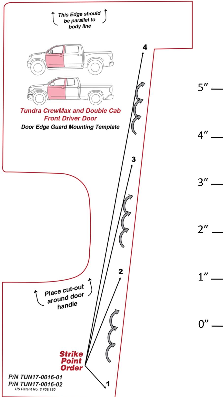
Dealer Installation Note: Check the above scale to ensure it is 1:1. Adjust on photocopier if it is not to scale. If this is a pdf document, set the "Page Scaling" to "None" in the Print dialogue box prior to printing.
