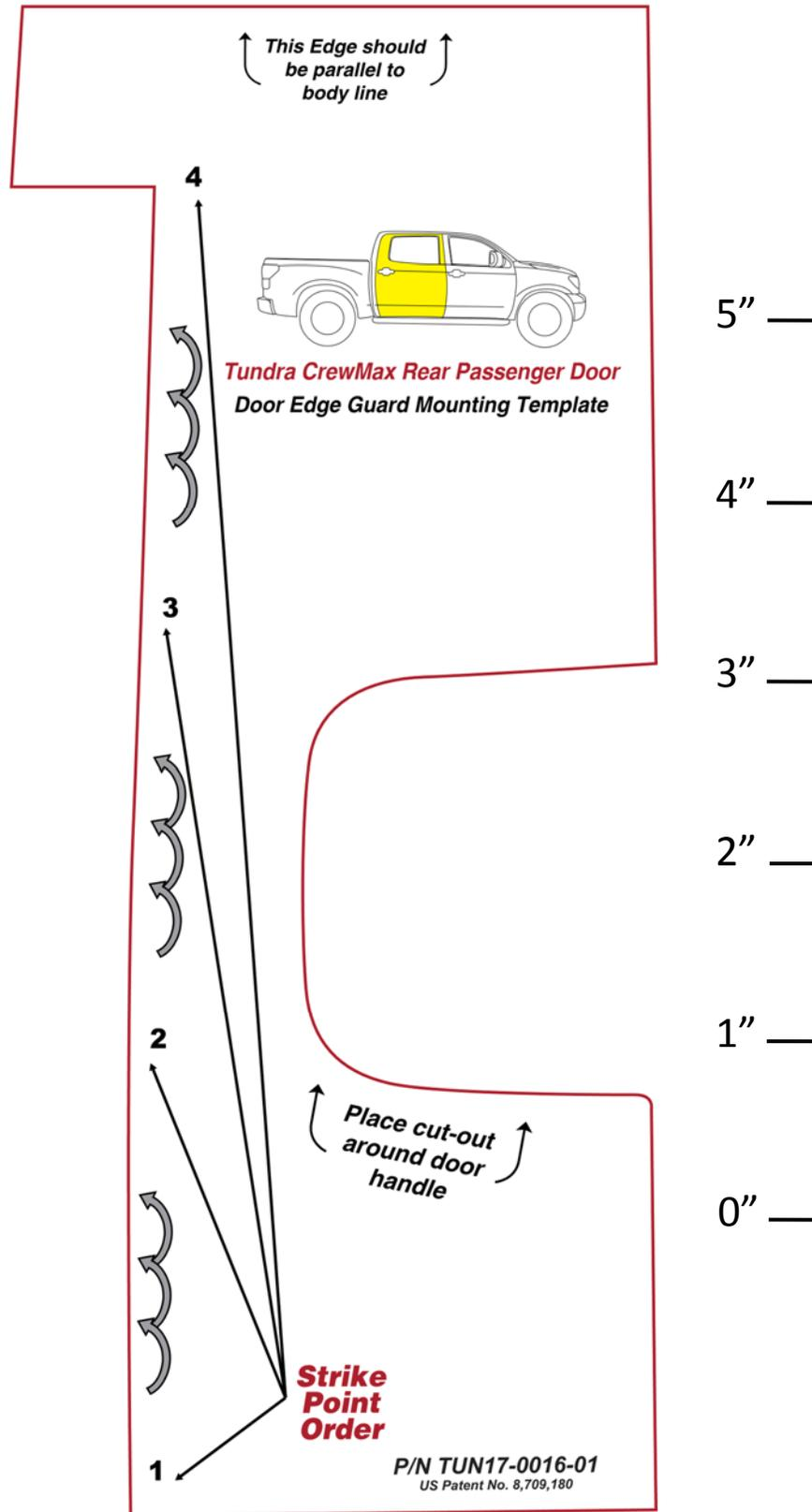
Dealer Installation Note: Check the above scale to ensure it is 1:1. Adjust on photocopier if it is not to scale. If this is a pdf document, set the "Page Scaling" to "None" in the Print dialogue box prior to printing.
