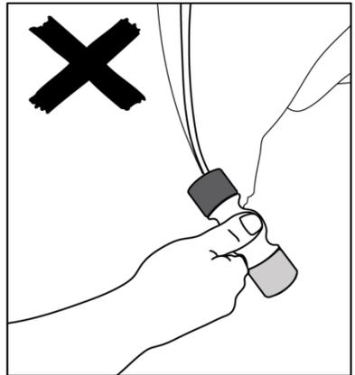
ENSURE MALLET HEAD IS PERPENDICULAR TO THE EDGE OF THE DOOR
