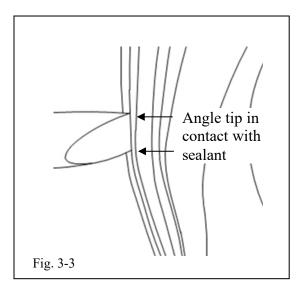
**ADJUST:** If sealant adjustment is needed then align the adjustment tool to the edge of the door, with the angle edge positioned toward the inside of the door (Fig. 3-3).
