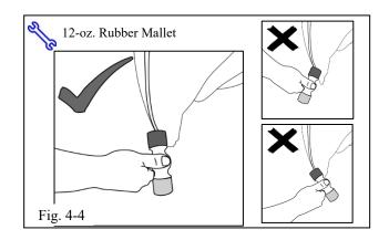
(1) Ensure the mallet head is perpendicular to the edge of the door (Fig 4-4).
