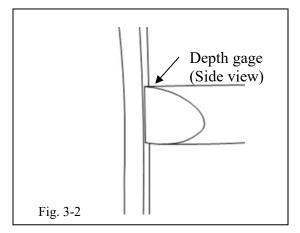
**GAGE:** Align the adjustment tool to the edge of the door, with the angle edge positioned toward the inside of the door (Fig. 3-2).
