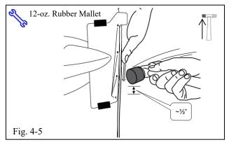
(f) Strike down the length of the door edge guard in ½" increments, guiding the door edge guard as you go (Fig 4-5).
