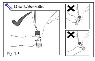
(1) Ensure the mallet head is perpendicular to the edge of the door (Fig 3-5).
