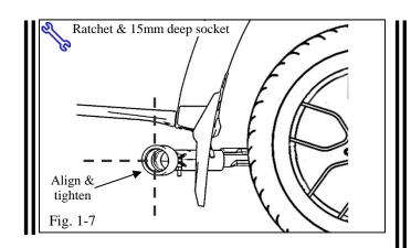
(g) Once the tip is positioned correctly and the alignment seems accurate, tighten the clamp nut making sure the bolt remains in a vertical 3 o'clock position (Fig. 1-7).
