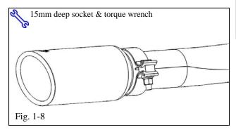
(h) Torque the clamp nut to 55 N-m (41 ft-lbf) (Fig. 1-8).
