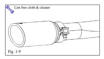
(j) Clean the exhaust tip with VDC approved cleaner (PPO) or glass cleaner (DIO) and a non-scratching cloth (Fig. 1-9).
