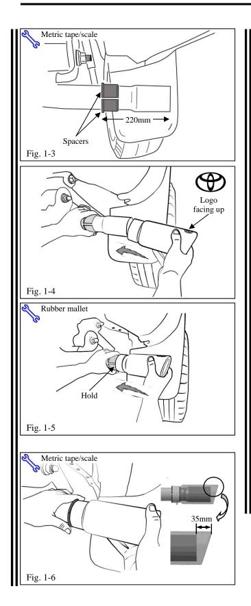
(d) Place the spacers on the exhaust pipe approximately 220mm from the tip (Fig. 1-3).
