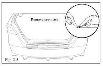
NOTE: It may be necessary to press down on the corner of the part as you roll back the premask.
