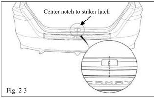
(c) Align the center notch directly below the striker latch opening and the leading edge of the pre-mask along the vertical surface of the bumper. Be sure not to roll the applique onto the vertical surface (Fig. 2-3).
