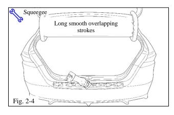
(d) Using long smooth overlapping strokes, squeegee from the center outwards of the horizontal surface (Fig. 2-4).
