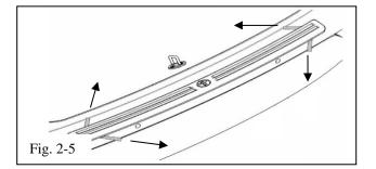
(f) Once the exposed tape has been secured, pull out and discard all the liners to allow full tape contact with the rear bumper (Fig. 2-5).
