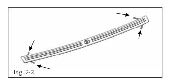
(b) Ensure all the tabs are folded so they can be accessed from the top once the protector is seated on the rear bumper (Fig. 2-2).
