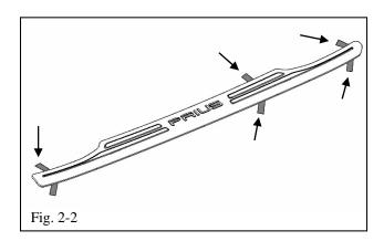
(b) Ensure all of the tabs are folded so they can be accessed from the top once the protector is placed on the rear bumper (Fig. 2-2).
