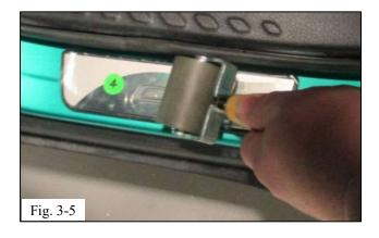
(d) Align the door sill against the curvature of the paper template and start bonding to the rocker (Fig. 3-4).
