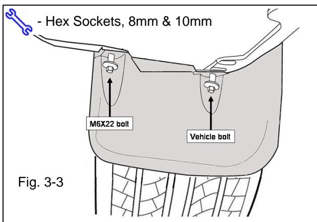
(d) Position the rear mudguard in place and secure it with the M6 x 22 bolt and the vehicle bolt removed in step 3.a. and then install the two #10 screws. (Fig 3-3 & 3-4)
