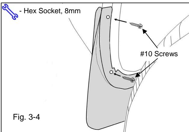
**NOTE:** When tightening the screws/bolts, push the rear mudguard onto the quarter panel to reduce the gap between the rear mudguard and the panel.
