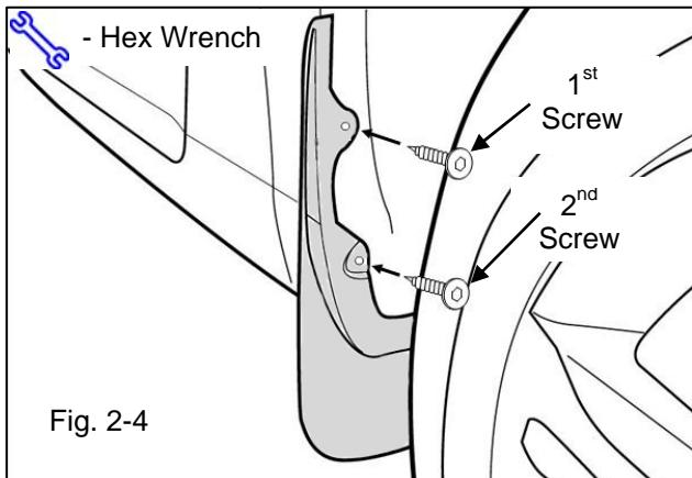
(d) Using the two screws removed in step 2-a, install the top screw first. Push mudguard tightly against fender and tighten. Then install the (2<sup>nd</sup>) lower screw. Push mudguard tightly against fender and tighten. (Fig 2-4)
