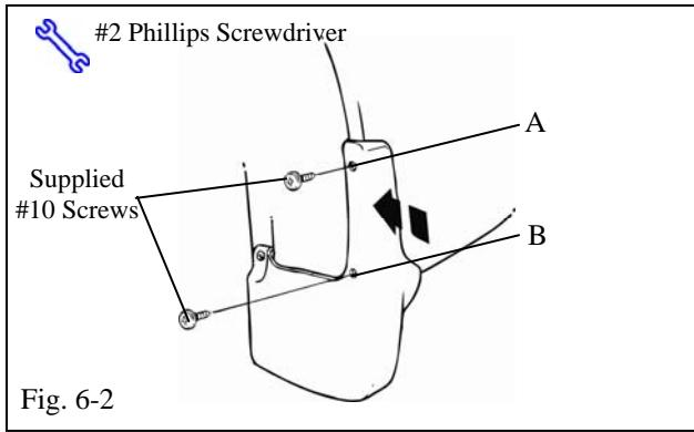
(c) Install supplied #10 screws in locations A and B while holding part up and tight against bumper panel. (Fig. 6-2)
