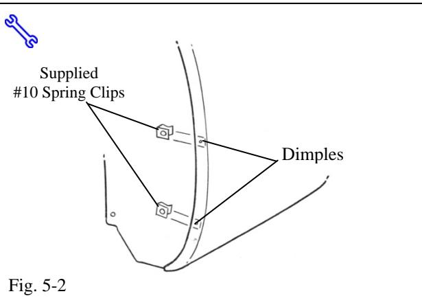
(b) Install supplied #10 spring clips over fender edge dimples with turned up edge on inside of bumper at locations A and B (Fig. 5-2)
