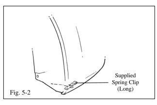
**(b)** Install supplied #10 spring clip (long) over fender liner with turned up edge on inside of bumper. (Fig. 5-2).
