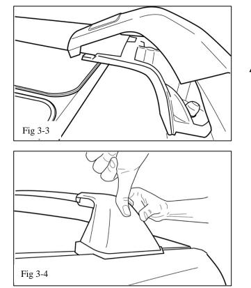
(b) Slide the top of the cover over the extrusion and snap the cover into place (Fig. 3-3 and Fig 3-4).
