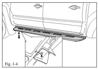
(d) By hand, place M6 bolts UP through the brackets into the threaded holes in the running board (Fig. 1-4). Start with the front position.
