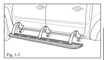
(c) Place the running board onto the brackets, aligning the front mounting location first (Fig. 1-3).
