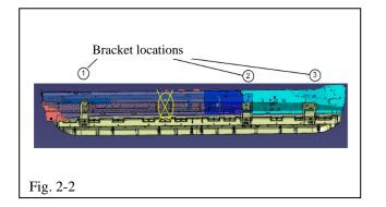
(c) Push up and align the two holes in the front bracket (location#1) to the weld nuts in the vehicle. Install and torque the two bolts to 19.5 N·m (14.4 ft·lbf) (Fig. 2-2).
