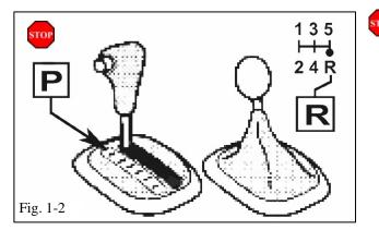
stor (b) Put transmission in "P" (automatic) or reverse (manual). (Fig. 1-2)
