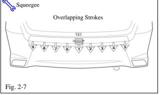
(f) Use long, smooth overlapping strokes with the squeegee from the center outwards of the horizontal section and begin to wrap over the bumper (Fig. 2-5).
