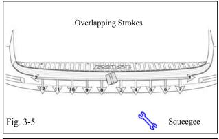
(e) Using long smooth overlapping vertical downward strokes squeegee from the center outwards of the vertical section (Fig. 3-5).
