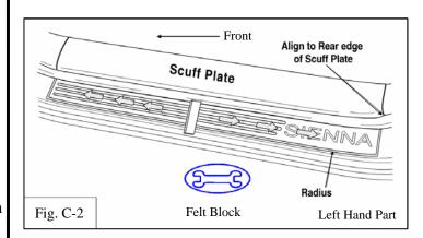
D. Installation of the Front Right Door Sill Applique.
