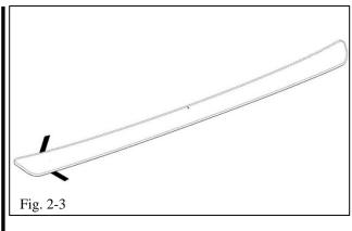
**NOTE:** Do not allow both ends of the protector to stick to the bumper before the center touches.
