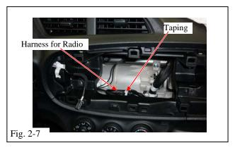
(e) Remove the taping on the harness for the radio unit. (Fig. 2-7)
