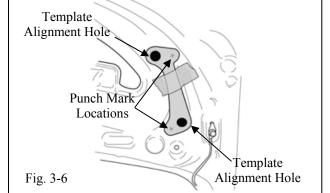
(j) Cut out the perimeter of the inner panel hole template and the two alignment holes. Place the template on the inner panel of the lift gate as shown on the passenger side. The alignment holes in the template will line up with existing holes in the inner panel. Center punch the two (2) punch mark locations. Turn the template over and repeat for the driver's side of the lift gate. (Fig. 3-6)
