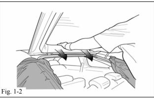
(c) Remove the trim panel across the inside of the lift gate window. (Fig. 1-2)
