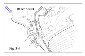
(i) Open the lift gate and disconnect the electrical ground on the driver's side of the inner panel of the lift gate and tuck it out of the way as shown. (Figs. 3-4 & 3-5)
