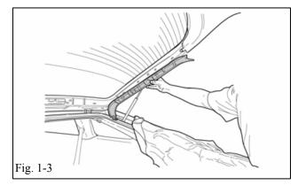
(d) Remove the LH and RH trim panels on the sides of the lift gate window. (Fig. 1-3)
