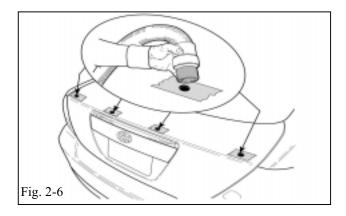
(j) Vacuum the surface of the trunk lid and the surrounding drilled areas and remove masking tape. (Fig. 2-6)
