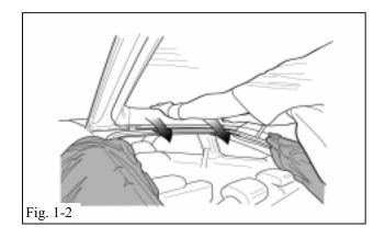
(c) Remove the trim panel across the inside of the lift gate window. (Fig. 1-2)
