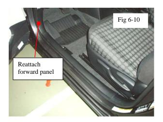
(i) Reattach forward rocker cover molding. (Fig 6-10)
