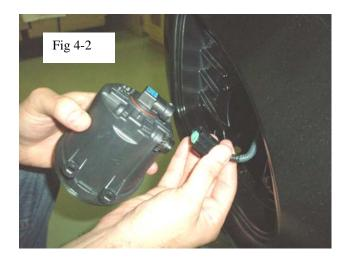
(b) Plug wire harness into fog lamp. (Fig 4-2)
