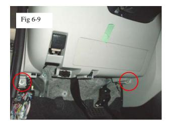
(h) Reassemble lower instrument panel and reinstall the two screws circled in Figure 6-9.
