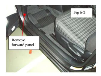
(b) After removing rocker cover, remove panel forward of the rocker cover molding. (Fig 6-2)
