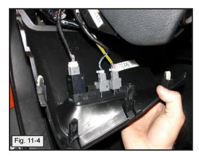
e. Disconnect all connectors and remove from vehicle. (Fig. 11-4)
