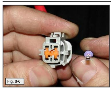
g. Insert terminal with purple seal from fog light harness into open cavity of turn signal connector. (Fig. 6-6)
