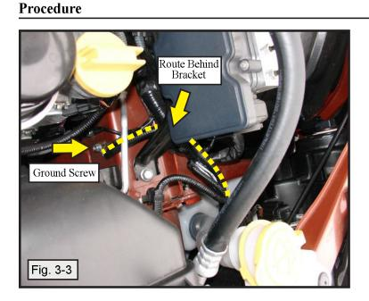
1. With the harness behind the bracket route harness towards driving light and down towards bottom of vehicle. (Fig. 3-3)
