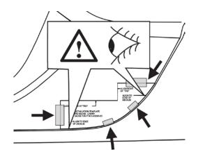
Remove liner from adhesive backing on "TRD" badge.
