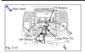
(r) Bundle the excess portion of the vehicle harness, then secure the V5 harness and vehicle harness with 1 large Wire Tie. (Fig. 3-15)
