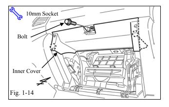
(v) Remove the glove box inner cover.
