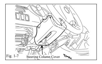
(m) Remove the lower steering column cover. (Fig. 1-7)
