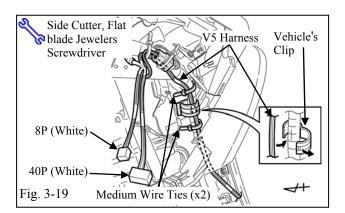
(w) Route and secure the V5 harness to the vehicle harness with two medium wire ties and the vehicle's wire clip. (Fig. 3-19)
