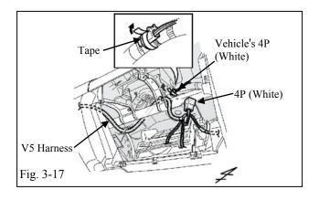
(u) Locate the vehicle harness' white 4P female connector and remove the tape securing the 4P connector. (Fig. 3-17)
