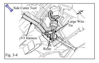
(d) Secure the V5 harness' relay to the vehicle brace with one large wire tie. (Fig. 3-4)
