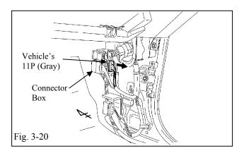
(x) Locate and disconnect the gray 11P connector to the connector block on the passenger side cowl area. (Fig. 3-20)
