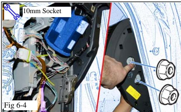
(e) Install the RES ECU as shown using 2 Nuts from the Kit. (Fig. 6-4)
