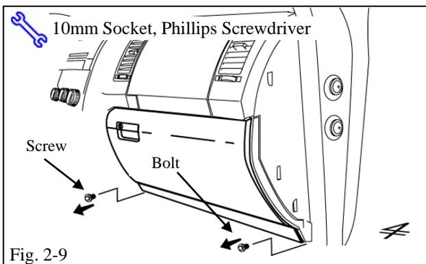
(k) Remove 1 Screw and 1 Bolt from the bottom of the Glove Box. (Fig. 2-9)
