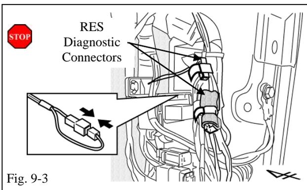
(c) Locate and remove the Tape securing the V4 Harness's WHITE 1P Connectors in the Passenger's Side Cowl Area and connect them. (Fig. 9-3)
