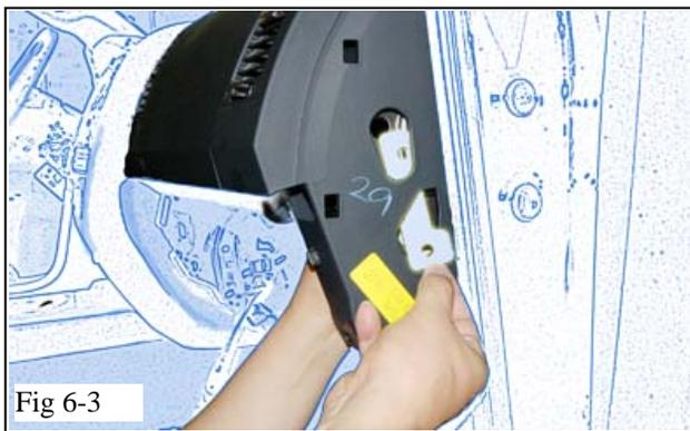
(d) Insert the V4 RES ECU Mounting Plate through the Hole on the side of the Dash. (Fig. 6-3)
