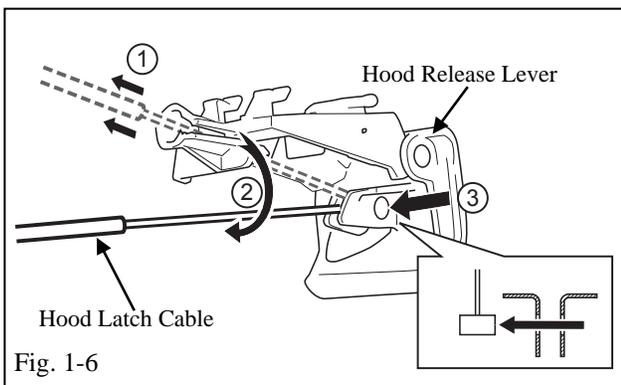
(f) Remove the Hood Latch Cable from the Hood Latch Lever. (Fig. 1-6)
