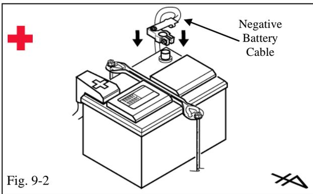
(b) Temporarily reconnect the Vehicle's Negative Battery Cable. (Fig. 9-2)
