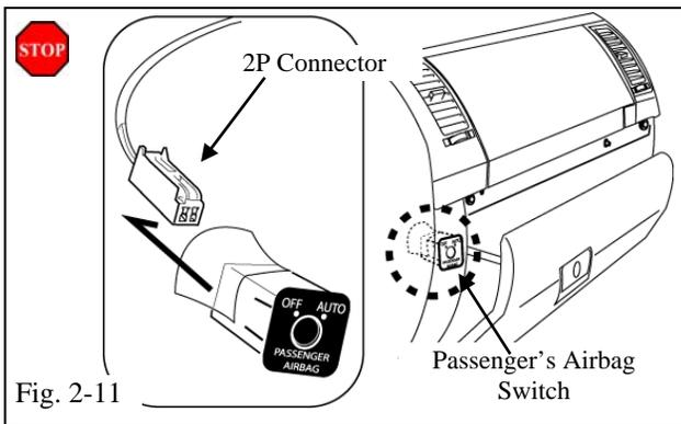
**FOR VEHICLES EQUIPPED WITH PASSENGER'S AIRBAG SWITCH (step m)**
