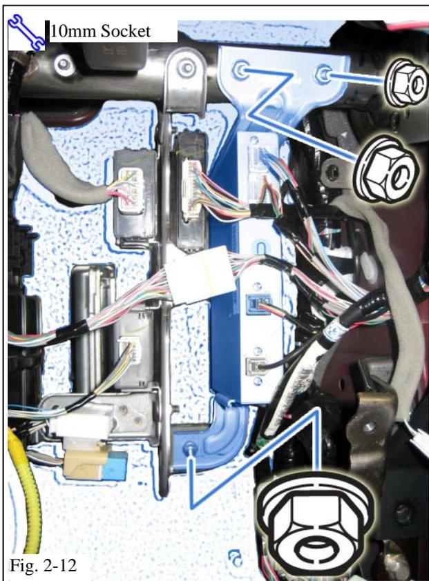
(n) Remove the Vehicle's ECU. (Fig. 2-12)
