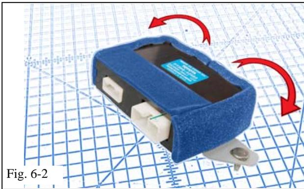
(b) Attach 2 pieces of Large Foam Tape to the sides of the RES ECU as shown. (Fig. 6-2)
